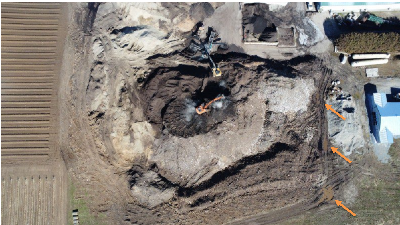
Photo 8. View of Leachate Discharge on the Southeast Side of the Facility (as indicated by the orange arrows).
